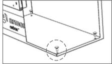
To install an OxBox in a vehicle, these instructions MUST be followed. The van boxes come with M10 bolt holes pre-drilled in the base of the box for fixing them down.
