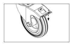
When the OxBox is stationary and in position, always ensure both castor brakes are engaged.
