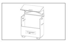
Only the OX3 and OX4 can be fitted with castors using the pre-drilled holes. Lift the box onto a stable platform. The box MUST be empty when fixing castors. Castors can be fitted to smaller boxes but holes will need to be drilled by the user.
