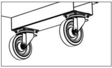
Repeat step two for the other wheels. Once complete, check all nuts are tight, and then ensure the two braked castors can swivel through 360° before lowering the OxBox.
