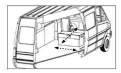
Once installed, test by pulling and pushing the box vigorously in various directions. It is imperative to ensure it is firmly fixed down.
