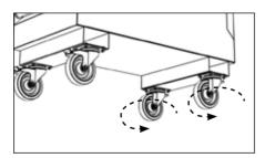
Armorgard castors kits come with two fixed and two swivel-braked castors. We recommend fixing the 2x fixed castors on the left and 2x swivel-braked on the right side of the box.
