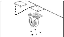
2. Insert castor plates into the fork-lift skids. Put the castor wheel in place and use a 13mm socket to tighten the M8 nylocks.
