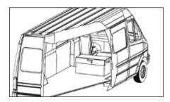
To install a TuffBank in a vehicle, these instructions MUST be followed. The installer must drill 4x 10mm holes into the base of the box, one in each corner, in order to fix it to the floor.
