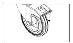
**3.** When the TuffBank is in position, always ensure the castor brakes are used.
