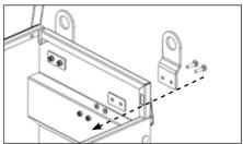
Thread the M10 coach bolts through the lifting eyes, then back through the box. Inside the box, add a backing plate, M10 washers and nylocks to each bolt as shown.
