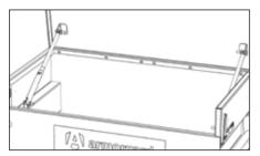
For the TuffBanks that can be fitted with castors, lift the box on to a stable platform. The box MUST be empty when fixing castors.
