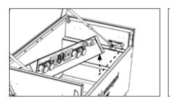
3. Slot the right hand side of the shelf down in front of the gas strut, bring it underneath and back up behind the gas strut.
