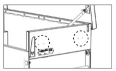
For the TuffBanks that can be fitted with crane lifting eyes, use a 10mm metal drill bit to drill out the four pilot holes located on each side of your TuffBank.
