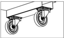
Repeat step two for the other wheels. Once complete, check all nuts are tight, and then ensure the two braked castors can swivel through 360° before lowering the TuffBank.
