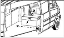
Once installed, test by pulling and pushing the box vigorously in various directions. It is imperative that it is firmly fixed down.
