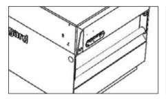
Always secure all locks and remove key before lifting the unit, to ensure that the lid does not open unexpectedly.
