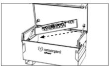
2. Slide the left end of the shelf into the TuffBank, under the gas strut with the SlamStop safety stay.
