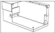
2. The TuffBank must then be fixed down using 4x bolts, washers and shear nuts. The TuffBank needs to have a bolt in each of its four corners, fixing it securely to the floor.
