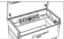
The shelf should now drop into place - depending on the model, this will either be on the lugs provided or onto the shelf created by the recessed handles.
