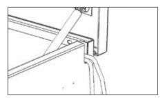
**3.** Up to two cables can be fitted through the cable passing point so a power supply and a tool can be fitted through simultaneously. The lid can then be closed and locked for secure charging.
